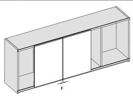
The centre reveal F between two wooden doors can be influenced by the position of drill holes B1 and B2 for the running and guide components. Use of the standard drilling pattern produces a centre reveal of F = 10 mm.
